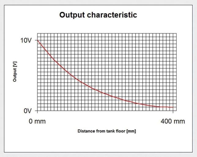
The Picture above depicts the analogue output volts related with the distance between the strip and the tank floor, considering 0 mm the tank floor (generally granite or marble domes).
